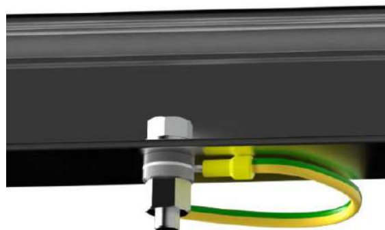
Fig. 11 Grounding of PV modules
